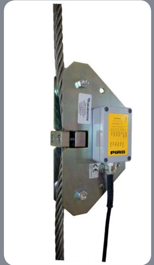
The LKVE is a force transmitter which is attached to a stationary rope part. The LKVE gives a 4-20mA output signal. It has high repeatability, is made for use in aggressive industrial environments and fully conforms to IP 67.
