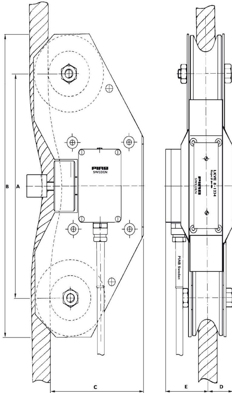
The drawing is for LKVE 8-12. The measurements for different LKVE capacities are shown in the table below. The other types are of a slightly different design.
